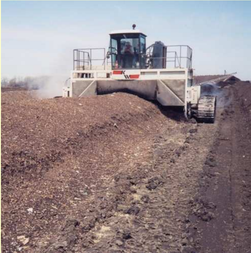
Turning a triangular windrow, source: RRSI Resource Recovery Systems International
